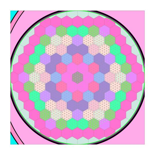
Serpent model used to calculate reactivity feedback coefficients
