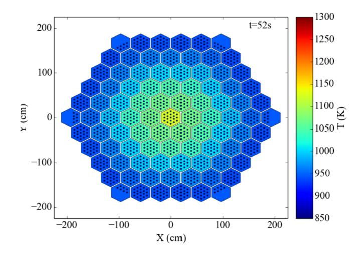
Example of CHD output (temperature distribution during transient)
