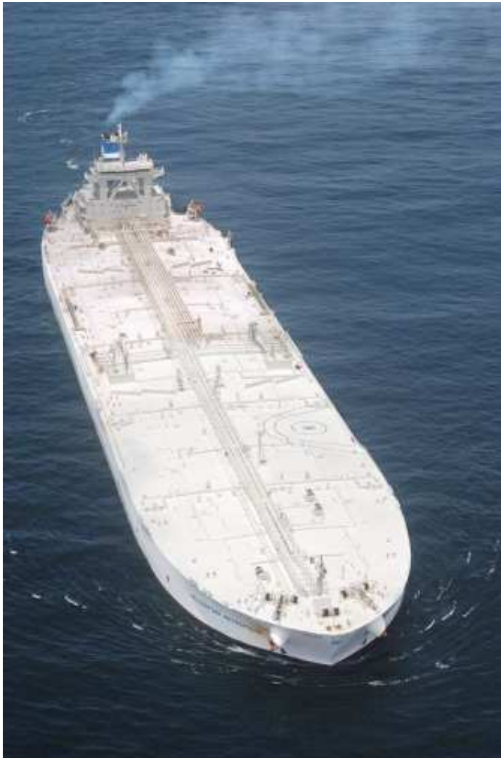
Figure 1: 440,000 ton tanker built in 1 year for $89 million
